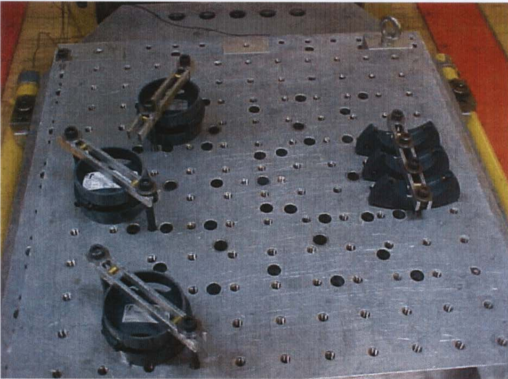
PHOTO 2 Vibration, random. Mounting of test specimens in Y-axis.
